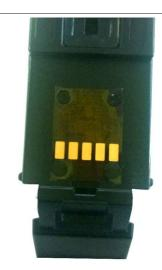
2) The photo to the right shows the cartridge after removal of the OEM chip and silicon.
