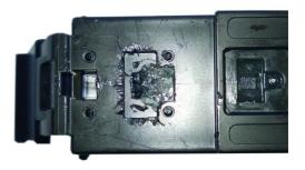
3) The highlighted area must be shaved (0.2mm - 0.4mm) down to reduce the thickness of the plastic. It's less than half a mm but it makes all the difference when installing the cartridge in the printer. Make a note of the lug/post positions before you shave them off.
