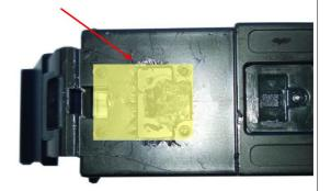
4) Photo of attached chip. It is recommended to test the cartridge in a printer to ensure the chip is correctly installed.
