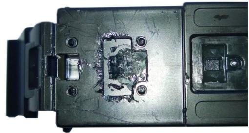
3) Locate the four posts again and apply a small amount of glue to each corner of the post. Next install the chip onto the four posts ensuring it is flat against the cartridge aligned correctly.
