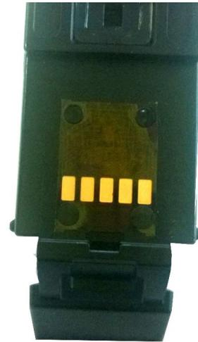
2) The photo to the right shows the cartridge after removal of the OEM chip and silicon. The replacement chip will not fit into the location if the majority of the existing silicon has not been removed.
