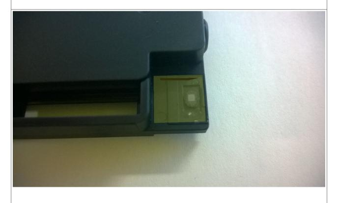
3) Photo of cut out area ready for chip placement. (Please note the square hole in the cutout is not required)
