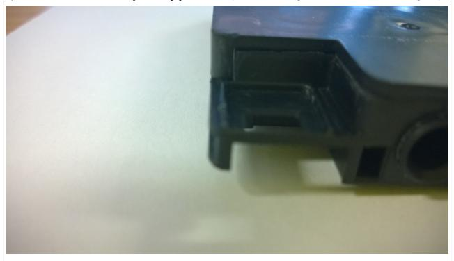
4) Photo of OEM HP932XL with Ausjet chip installed after the cartridge has been modified.
